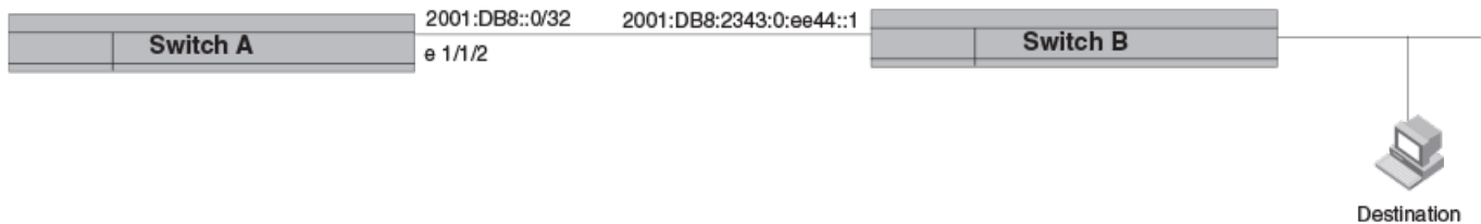
FIGURE 18 Example of a Static Route
